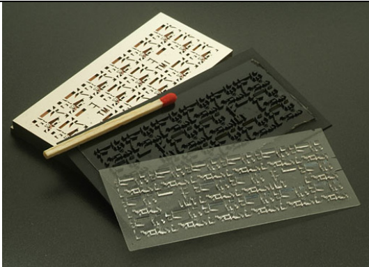
Large micro structured area produced by hot embossing.
